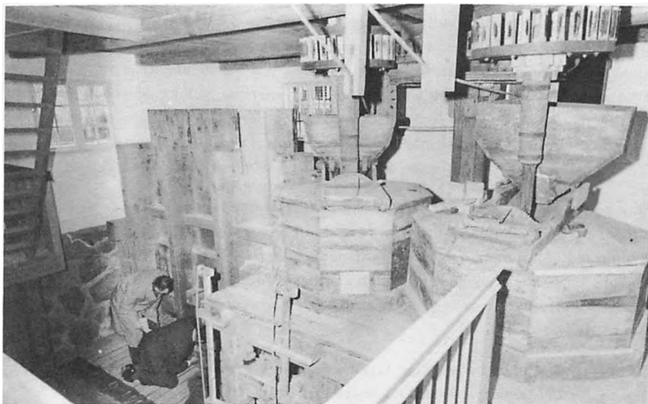
Fig. 21; neg. 1768.32; 08-05-65; Det færdige stampeværk i funktion. Completed plant in operation. The lintel over the fulling frame still missing.
