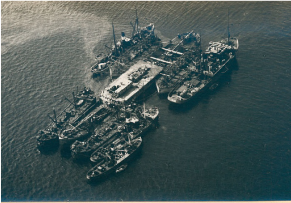
M/S »ESBJERG« salvaged by wreck-raising pontoons in the Baltic during the summer 1946.
